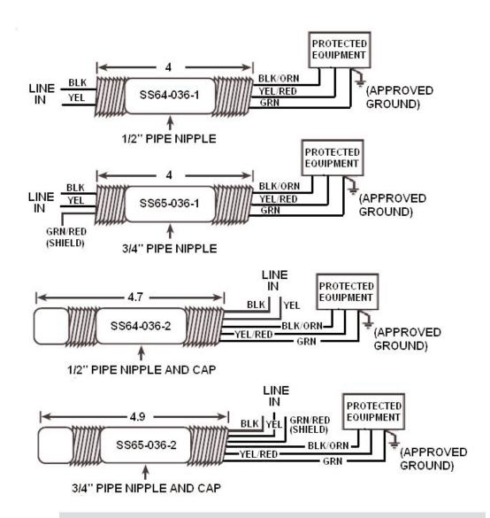
**Caution:** The hybrid design of this product includes series resistance. Do not place this product in service on any signal lines capable of supplying more than 150 milliamperes continuously.
